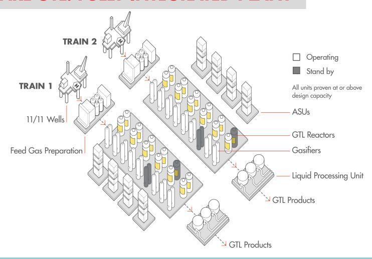
DESIGN CAPACITY: 1.6 BCF/D OF WET GAS
